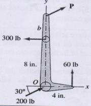
3- I f P =20 N, replace the three couples with a single equivalent couple, specifying its magnitude and the direction of its axis
